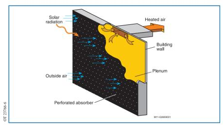
With the exception of the fans, the transpired collector has no moving parts and requires no maintenance.
