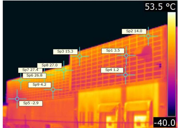
perforations in the Lubi collector near the fans but not through perforations some distance from the fans. These results are consistent with a pressure drop below 25 Pa and a Lubi system operating below the tested and rated flow rate of 4 cfm/ft<sup>2</sup>.
