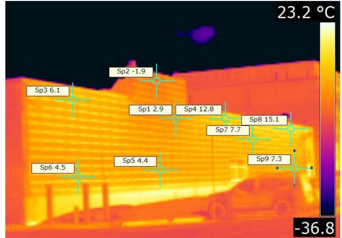
The above IR image of the entire Lubi Collector shows uniform air flow under and to the left of the fan but shows a hot section along the top right side. The next IR image depicts the right half of the Lubi collector and clearly shows the top portion to be 10 to 16 C° warmer than the Lubi collector near the fan.
