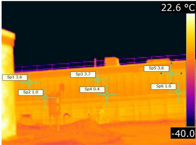
With over 5000 cfm of incoming air and a centrally located wall intake, the flow rate is over 6 cfm/ft<sup>2</sup>. The uniform temperatures and no hot spots (a variance of 2 to 4 C° from bottom to top is normal) indicate that air is entering through each perforation to cool the entire surface and that the 25 Pa pressure drop is likely being maintained across the collector.
